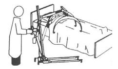
**10.** Disengage support hoop hooks from stretcher support bars. Raise boom to clear patient. Release brakes and remove scale from bedside. Remove stretcher from under patient.
