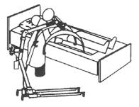
5. Move scale to patient's bed. Open base legs to maximum OPEN and LOCKED position (for maximum stability), and then set brakes on rear wheels. **6.** Lower boom until stretcher support hoop hooks reach mattress and attach stretcher support bars to support hoop hooks.
