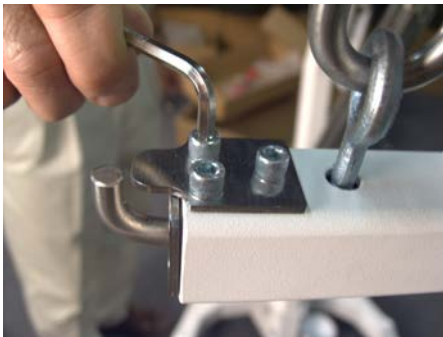
Remove outer 2 Screws Loosen inner Screw
