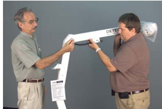
Have an assistant hold the Boom Assembly while inserting the bolt
