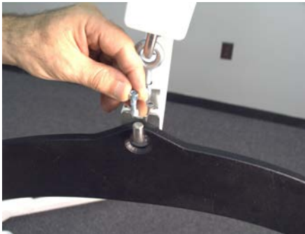
Lift hoop slightly to ease screw installation
