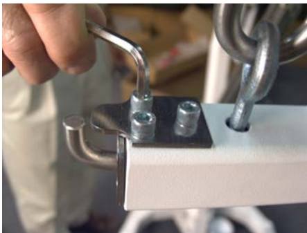
Remove outer 2 Screws Loosen inner Screw
