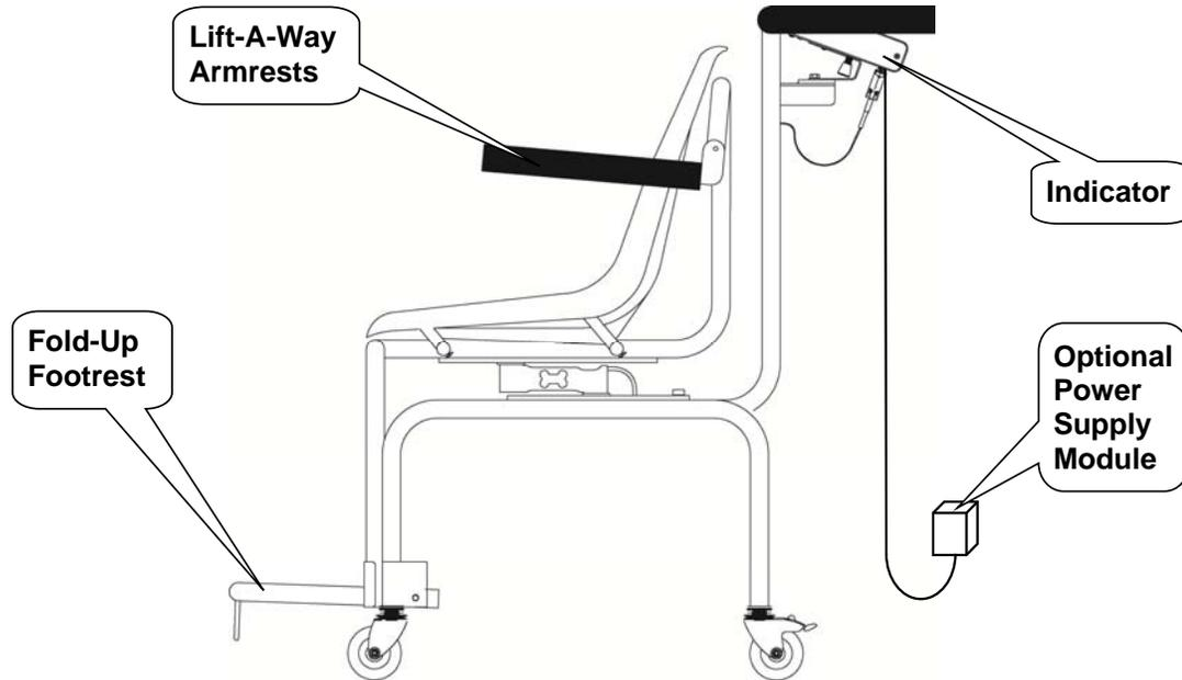
1. Install six (6) "AA" size batteries or if ordered with the scale, plug the small connector end of the power supply cord into the power jack located in the bottom right corner at the back of the indicator, then plug the power supply module into an appropriate power receptacle. **NOTE!** DO NOT connect a power supply to the indicator if alkaline batteries are installed.
