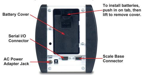
1. Obtain and install six AA alkaline, Ni-Cad, or NiMH batteries or if a -AC model, plug the small connector end of the AC power adapter cord into the AC power adapter jack located in the bottom right corner at the back of the weight indicator and then plug the AC power adapter into the proper electrical outlet.
