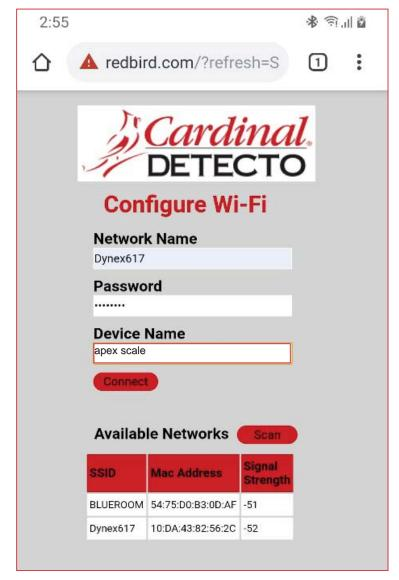
Enter the Network Name (SSID), Password, and Device Name (optional) for the network you wish to connect to. Note that the Device Name can be anything. Click on the **Connect** button and the module should try to connect to that network. This may take several seconds. The module will store these network credentials and connect to this network each time the scale is turned on.
