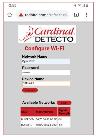
Enter the Network Name (SSID), Password, and Device Name (optional) for the network you wish to connect to. Note that the Device Name can be anything. Click on the **Connect** button and the module should try to connect to that network. This may take several seconds. The module will store these network credentials and connect to this network each time the indicator is turned on.
