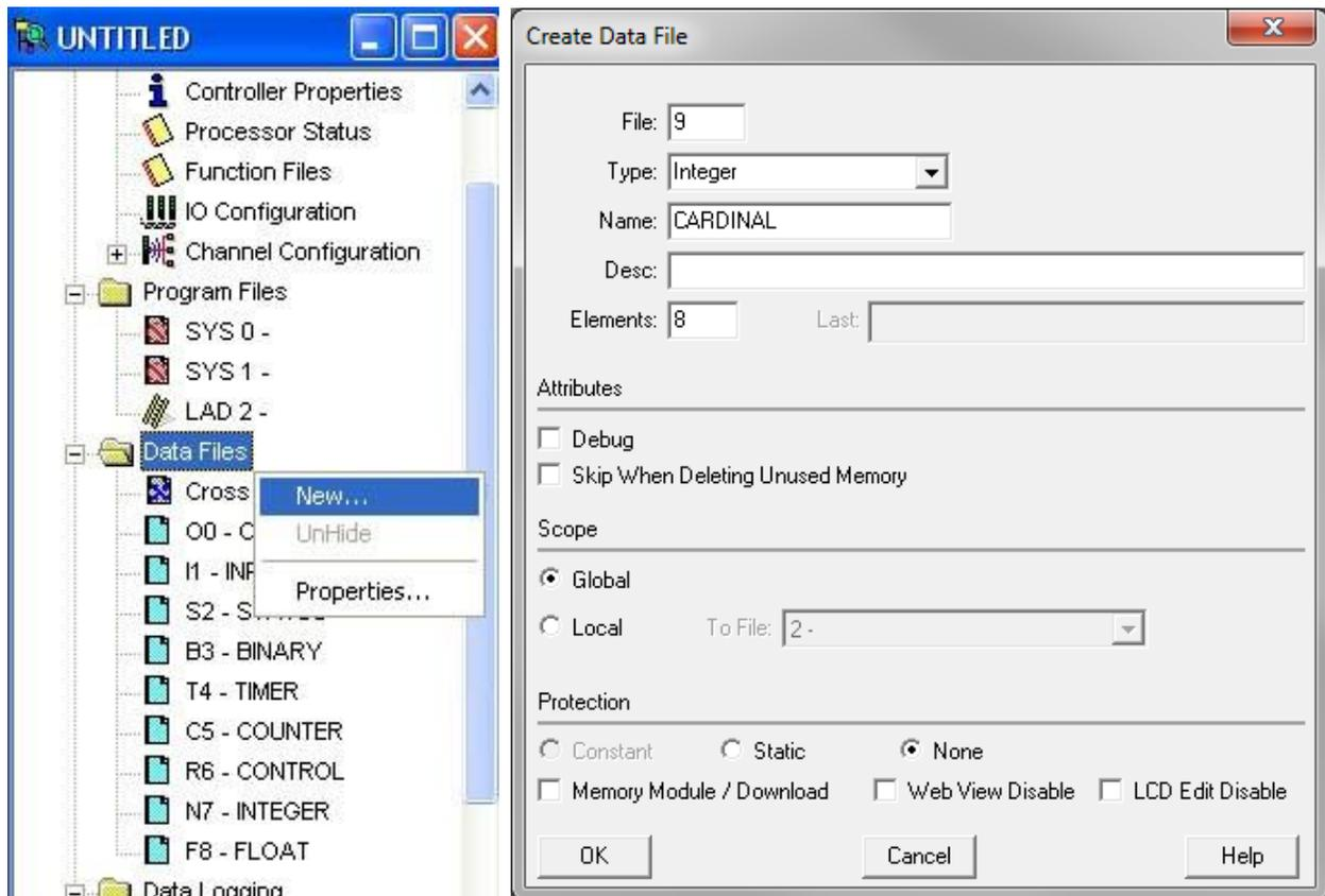
Next, create a data file for Message Type that contains 2 elements, one to control the Read Instruction and one for the Write Instruction. Create a data file for Extended Routing Information with 2 elements to store the information from the message instruction.
