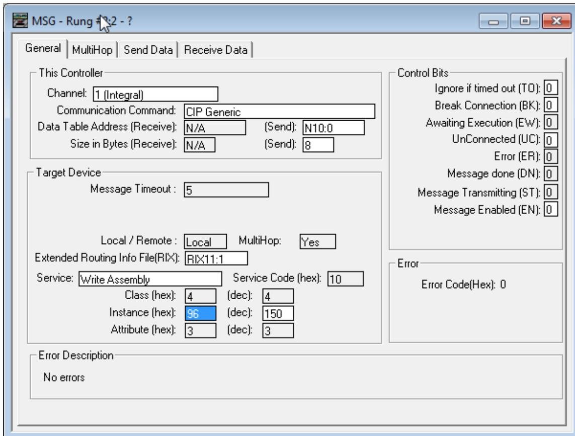
Next, select the “MultiHop” tab and type in the IP address of the 201. Under the “Send Data” tab will be the data that gets sent from N10:0 to the 201.
