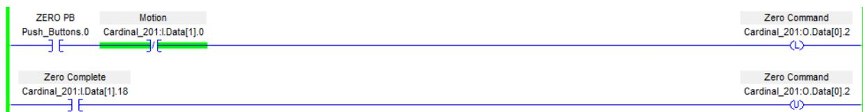
All of the commands bits should be processed like the example for the zero command except for bit 4 and 8. When the KB Tare command is processed it will need a floating point or decimal value copied into Word 1 for the Scale Tare Weight value. Then bit 4 can be processed like the other command bits. Bit 8 requires four bits of outputs to be specified starting at the third byte (bit 16) of Word 0.
