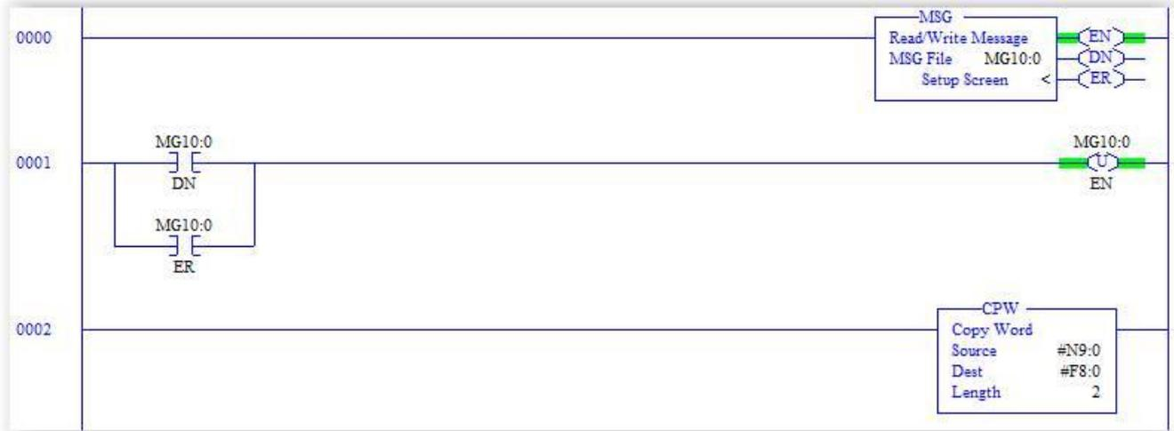
To read continuously from the 201 the MG10:0/EN bit will have to be unlatched after the MG10:0/DN is complete. This will retrigger the MSG instruction to start the read from the 201 again. ORing the MG10:0/ER bit will discard a message transfer error and unlatch the enable bit, thus retriggering the transfer.
