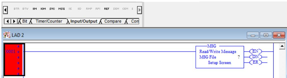
Select the Setup Screen inside the MSG box. Select Channel 1 for the controller. Use the pull down menu to select “CIP Generic” under the Communication Command.
