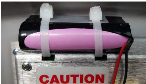
CORRECT! Position Cable Ties Connection on Top of Batteries.
