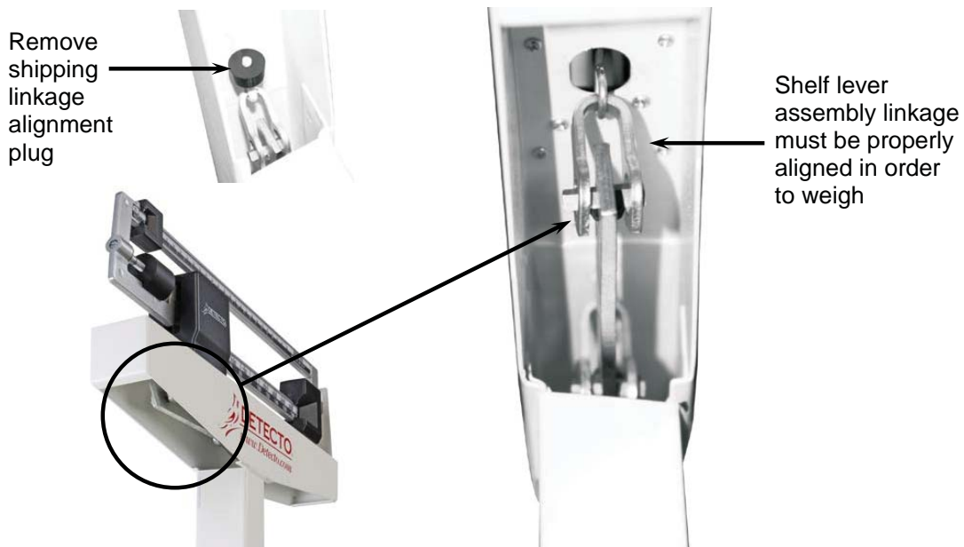
Figure 2. - View of linkage underneath weigh beam headpiece
