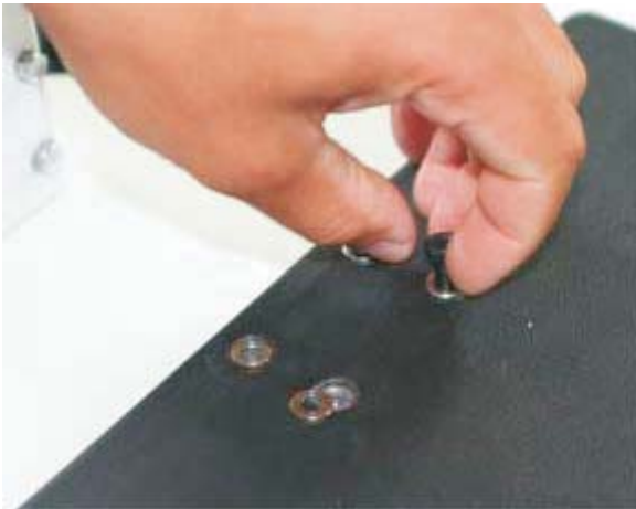
Figure 10. - Remove the four hex head screws from scale platform
