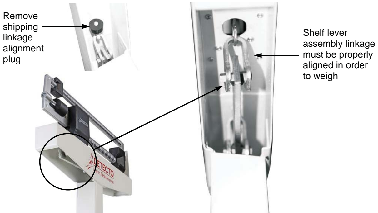
Figure 6. - View of linkage underneath weigh beam headpiece
