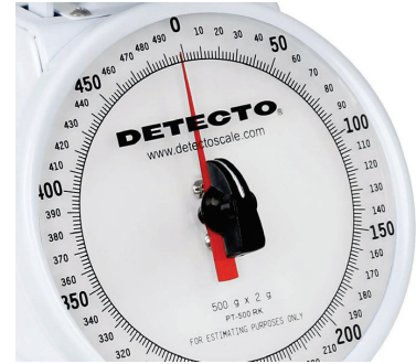
Turn Zero Adjust Screw until pointer is at '0'
