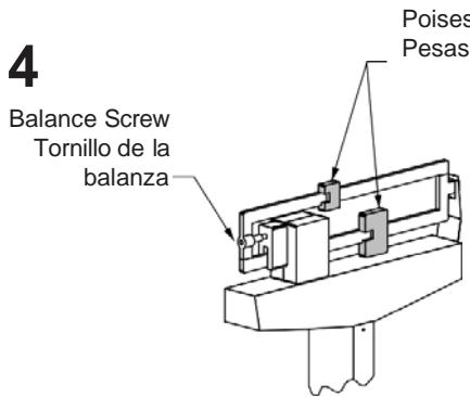
To balance scale, move both poises to zero (0) and turn balance screw to right or left until scale balances. For accurate weighing, place scale on level floor.
