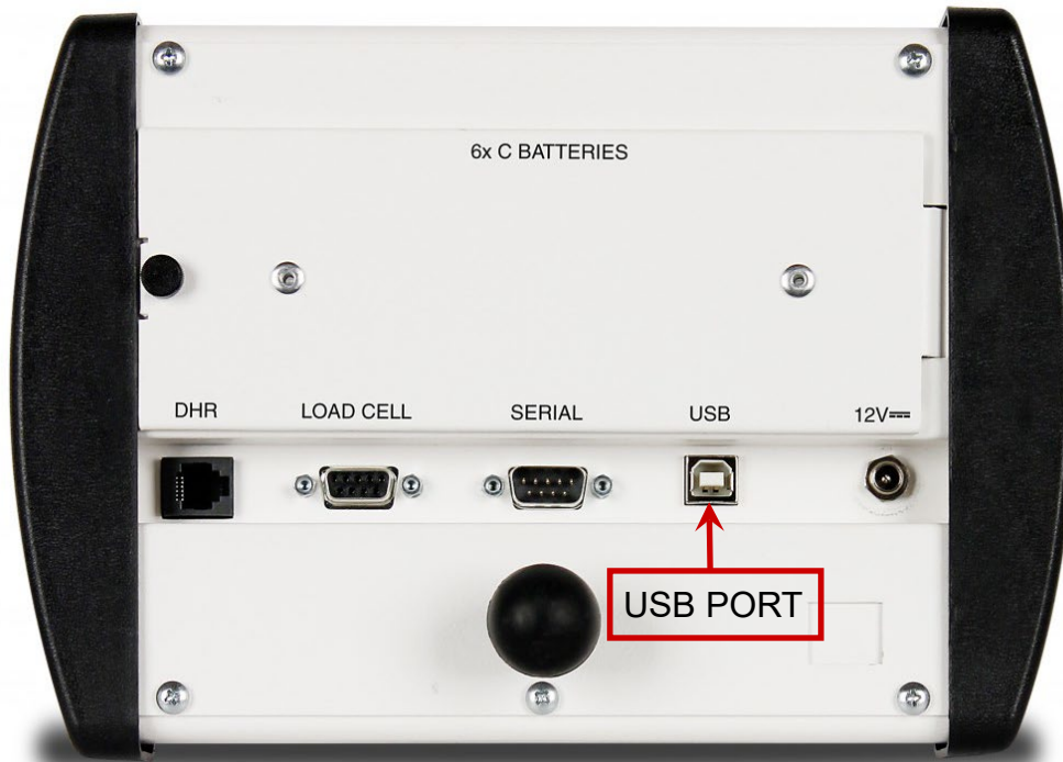
Location of USB port on back of MedVue
