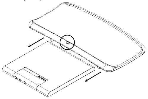
2. Turn scale upside down to screw tray and platform together properly.
