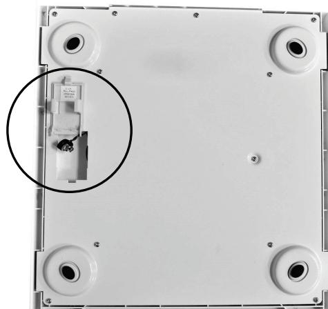
3. The scale uses a 9V alkaline battery.
