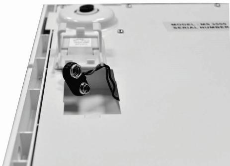
4. Install the 9V alkaline battery.
