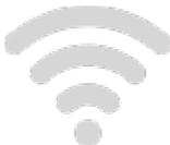
This display annunciator indicates a Wi-Fi network is available, but the cart is not connected to it.
