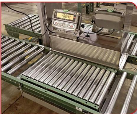
*The filled cherry container then proceeds down the conveyor line to the checkweigher, comprised of a Cardinal Scale EB-150-LPAN with 190 Storm washdown indicator.*
