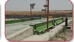
"Cardinal Scale's authorized dealer, Traffic Tech, assisted with the project using Cardinal Scale's load cells, two SB500 remote displays, an unattended 825 indicator in conjunction with Traffic Tech's weighbridge, camera system, printer, and RFID for driver identification."
