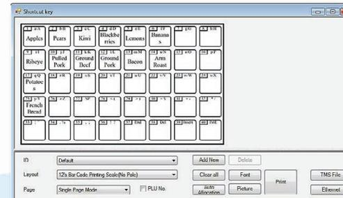
This graphic display allows PLUs to be quickly assigned to quick keys. This page can then be printed and used as the quick key overlay for the DL Series scale.
