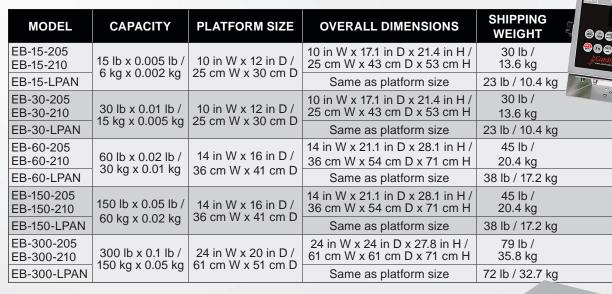
Select the size and capacity scale that you need and match it up with the Cardinal Scale weight indicator that best suits your application. The 205 indicator is great for basic weighing and the 210 indicator has additional features like keypad tare, piece count, and checkweighing.
