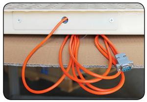
Scale is now ready to connect to digital weight indicator and calibrate.
