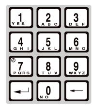
**NOTE:** The  $\mathbf{0}$ ,  $\mathbf{1}$ , and  $\mathbf{7}$  keys have dual functions. They are used to enter numeric data during setup and calibration as well as during normal operations. In addition, the  $\mathbf{0}$  and  $\mathbf{1}$  keys are used to select no (0 = NO) or yes (1 = YES) to various prompts.
