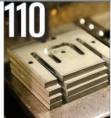
The icon's load cell bodies are stamped out with 110 tons of force. The load cell bodies are constructed of aircraft quality aluminum for maximum longevity and durability.
