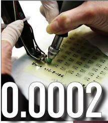
The origin of weight in every DETECTO icon® physician scale begins on a microscopic level with the strain gauge. Every icon® strain gauge is constructed with a foil sensor that is 0.0002" thick.
