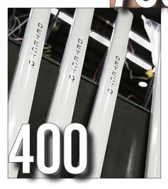
Each icon® column is prepped and painted with the highest quality powder coat paint. From start to finish, an icon® column can be completely painted and cured at 400° Fahrenheit in 60 minutes.
