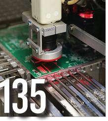
DETECTO's surface mount technology electronics machinery produces its own circuit boards in-house from American and foreign components. 135 components are added to each raw board before it is placed in the indicator. Each individual circuit board takes 150 seconds to complete on the SMT machine.
