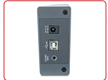
USB port for weight data transmission to an electronic medical records system
